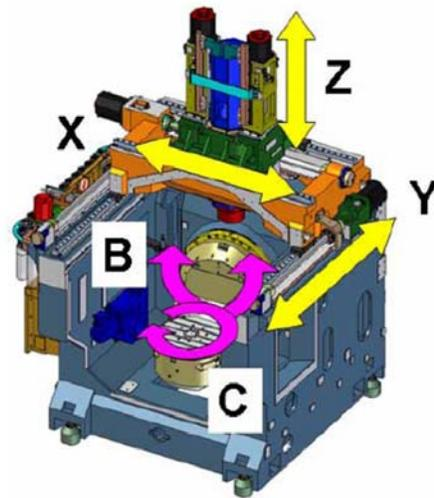
Fig.2 Outline of Structure of 5-axis machining centers(DMG Mori Seiki, NMV5000)with table-on-table type
