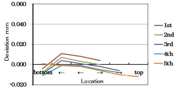
(c) Rotating motion and simultaneous 2-linear-axis control machining (Right gear tooth)
