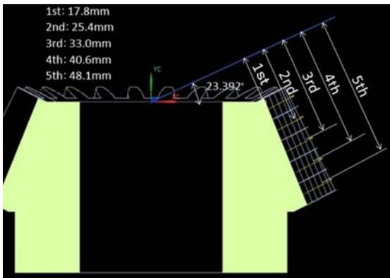
Fig.5 Measured points of machined deviation of bevel gear
