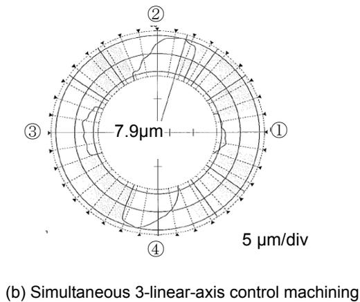
Fig. 8 Out-of-circularity of the machined cavity cone with grooves (measured at the position with 45 mm high from the bottom )
