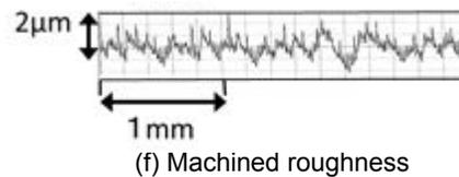
Fig.9 Machined profiles along the line of the cavity cone with complex geometry
