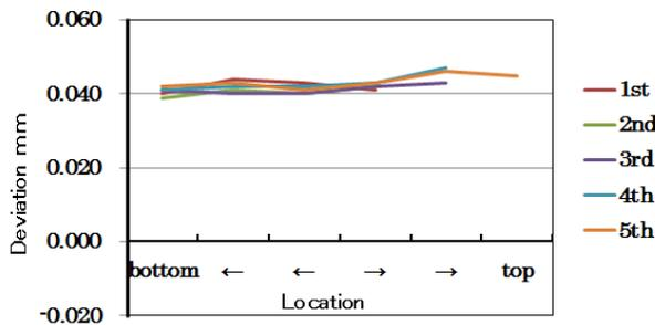
(b) Simultaneous 3-linear axis control machining with ball end mill (Left gear tooth)
