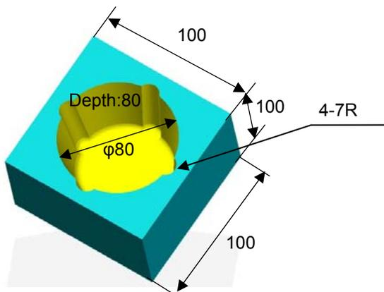
(b) Cavity cone with grooves
