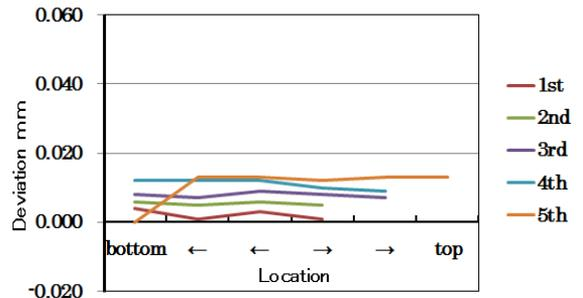
(d) Rotating motion and simultaneous 2-linear-axis control machining (Left gear tooth)
