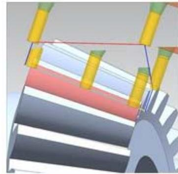
(Pattern 2) 5-axis control machining with square end mill
