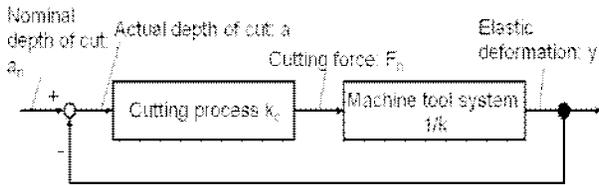
Figure 3: Static cutting process as a closed loop system.
