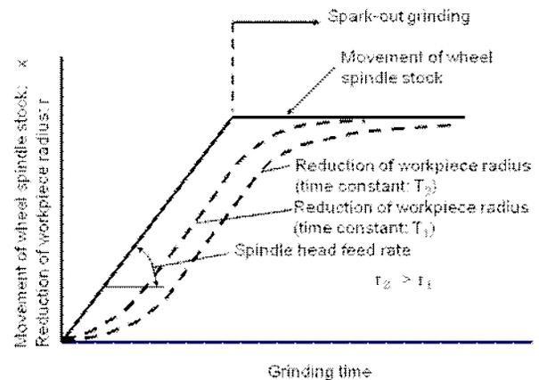
Figure 5: Grinding process as the first order time delay system.
