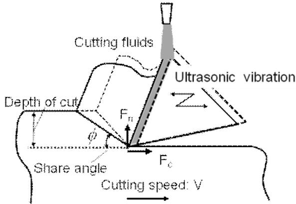
Figure 6: Effect of ultrasonic vibration in cutting.
