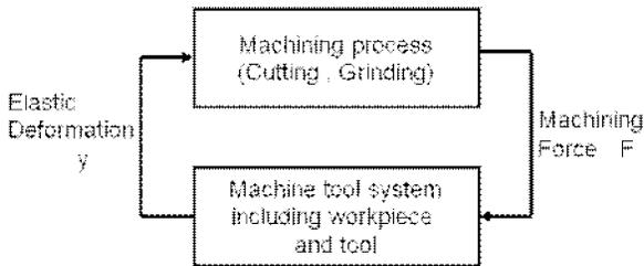
Figure 1: Machining process as a closed loop system.
