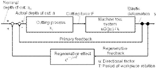
Figure 8: Dynamic cutting process.
