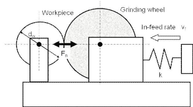
Figure 4: Cylindrical plunge grinding process.
