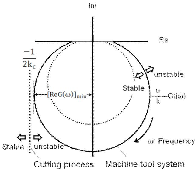
Figure 10: Vector locus of dynamic cutting process.
