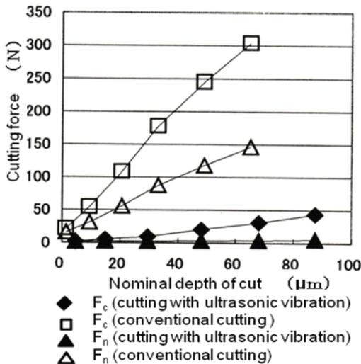
Figure 7: Reduction of cutting force by ultrasonic vibration.
