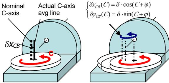
(a) Position error of C-axis avg. line,  $d_{XCB}$ .
