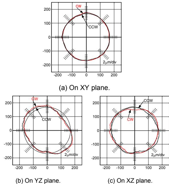
Figure 5: Circular test error profiles measured by DBB5.
