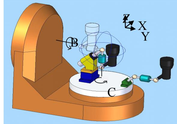
Figure 4: Configuration of the modified DBB device, DBB5
