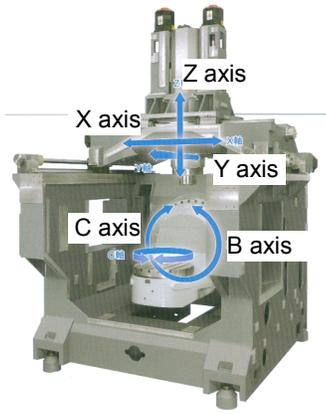
Figure 1: Configuration of experimental five-axis machining center [21]
